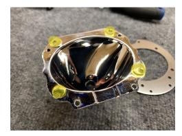
The wires for the bi-xenon motor will pass through a hole that is in the adapter plate and through the reflector bowl edge. The wires come with the pins already installed for the 9005/9006 connector. You are welcome to try and feed the pins through the hole one at a time, I found it faster and less frustrating to clip the wires and then use butt connectors to splice them back together.
