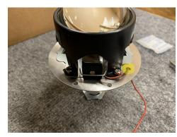
And on the backside. Once installed, you will want to put a dab of sealant over this hole and around the wires to seal it.
